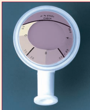
Color indications on detector dome
